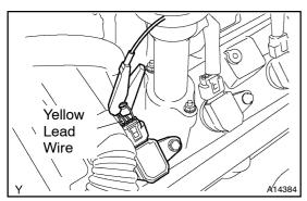
(b) Connect the tester probe of a timing light to the yellow lead wire of the ignition coil connector for No.1 cylinder.
