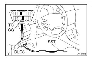
(c) Using SST, connect terminals TC and CG of the DLC3. SST 09843–18040
