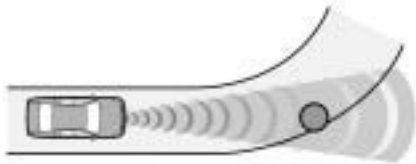
Object on road surface at corner entrance (Guard Rail, Street Light, Sign, Signboard)
